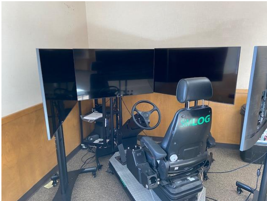
Simulator will full chair, steering wheel, 4 levers, 3 forward screens and 1 reverse screen
